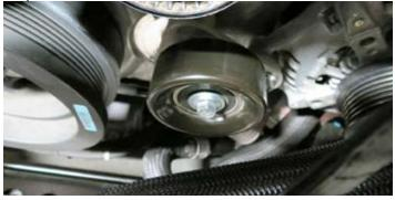
48. Verify that the tensioner is clocked correctly by sliding the index through the hole on the bracket. Install the supplied belt around the tensioner pulley and torque the M10 bolt supplied in Bag # 2 with a 15mm socket to 32 ft-lbs.
