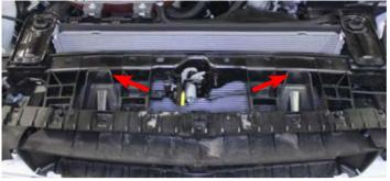
83. In front of the radiator, undo the lower shutter actuator arm by removing the two (2) bolts pictured. Swing out of the way and pull the shutters out through the front of the vehicle.
