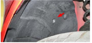
9. Reaching through the shown opening, remove four (4) nuts, two per side, securing the fascia to the fender using a 10mm socket.
