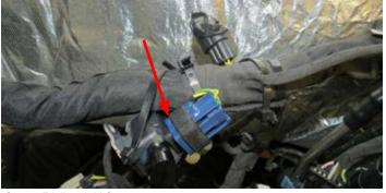
©2019 Edelbrock LLC Part #15832, 158320 38. Tape up the end of the two (2) IMRC position sensor plugs and secure plugs to the main harness out of the way. These will not be reused.
