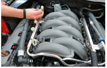
31. With the vehicle **COMPLETELY** cooled. Put rags under the fuel rail fitting and remove the fuel line from the rail. Cap off the fuel rail and fuel line with appropriate cap and plug to prevent spillage. Clean up any spilt fuel before proceeding.
