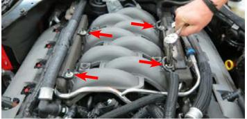
29. Remove the retaining brackets and the foam insulators from the fuel rails.
