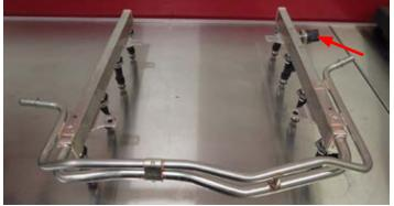
61. Apply fuel resistant thread sealer to the threads of the fuel pressure sensor adapter. Thread the adapter into the supercharger fuel rail until snug. **Ensure not to overtighten and strip threads.** Apply the same thread sealer to the fuel pressure sensor and thread it into the adapter. Prevent the adapter from twisting in further with a second wrench. Optionally continue to twist the sensor once snug until it aligns with fuel rail.
