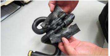
77. Remove the hose that attaches to the check valve and replace with the supplied 3/8" hose. Attach the supplied vacuum cap to the opposite end of the aspirator.
