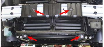
82. Remove the two (2) clips securing the shutter bracket to the core support.
