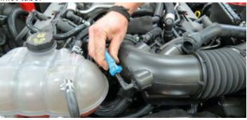
20. Disconnect the brake aspirator hose from the manifold PCV hose.
