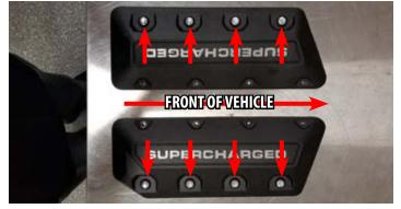
133. Place the evap in position for the coil covers. TIP: Place the bolts through the coil covers first, then feed the bolts into the evap bracket. Then thread the bolts into the supercharger coil cover brackets.
