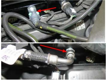
69. Reinstall the passenger side heater hose fitting using the factory hardware.
