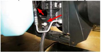
14. Remove the front strut tower brace (if equipped) using a 15mm socket. **NOTE:** The brace will not clear the supercharger manifold and cannot be used. The bolts securing the brace can be reinstalled once the brace is removed.
