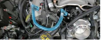
27. Disconnect the throttle body connector.
