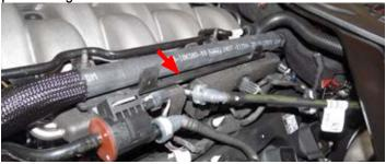
32. Repeating spill protection procedures from step 46, remove the fuel line from the passenger side fuel rail. Use a 3/8" fuel line disconnect tool to remove the line.
