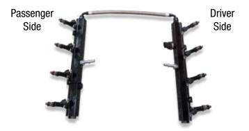
58. Apply O-ring lube to both ends of the original fuel injectors, then install them into the supplied fuel rails. Orientate the electrical connectors to face away from the supercharger.
