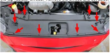
4. Remove six (6) bolts securing the top of the fascia using an 8mm socket.
