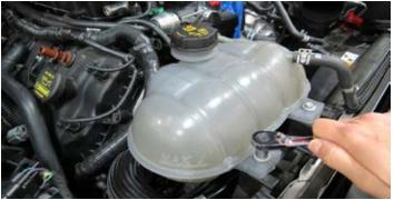
75. Install the supplied coolant bleed hose and secure with the factory hose clamps.
