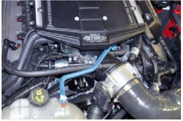
76. Carefully remove the protective foam from the brake aspirator.
