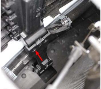
84. Remove the crash beam cross braces, if equipped.
