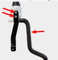
94. Connect the Water pump to Surge tank hose to the water pump and secure with a hose clamp from Bag #3.
