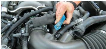
18. Remove the driver side PCV hose from the air inlet tube.
