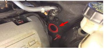
26. Remove the passenger side PCV hose from the valve cover and the intake manifold.
