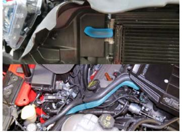
93. Attach the surge tank bracket to the surge tank using two (2) M6 x 10mm bolts from Hardware Bag # 3. Also attach the water pump hose to the surge tank and secure it with a hose clamp from Bag #3.
