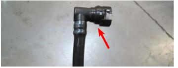
98. Attach the  $90^{\circ}$  fitting onto the supplied 1/2" Cadbar hose. Connect the quick connect fitting to the passenger side valve cover and the other end of the hose to the barb on the supercharger nose.
