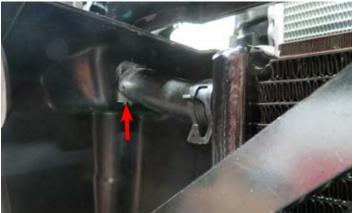
89. Attach the LTR to WP hose to the water pump and secure with a hose clamp from Bag # 3.
