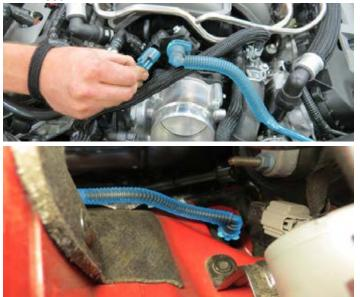
23. Using a hose clamp tool and pliers, remove the brake aspirator hose from the intake manifold.
