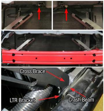
87. Using a drill and a 1 1/4" hole saw bit, drill a hole in the shroud that lines up vertically and parallel with the lower LTR barb.
