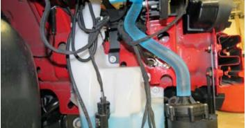
95. Secure the Surge Tank to Manifold hose to the surge tank and manifold using two (2) hose clamps from Bag # 3.
