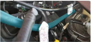
80. Route the Aspirator to Manifold hose under the heater hose and attach to the fitting on the supercharger nose.
