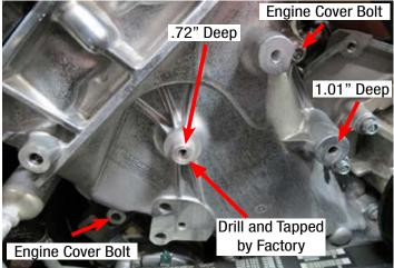
43. Secure the new tensioner bracket to the bosses that were just drilled and tapped with bolts supplied in Bag # 2.
