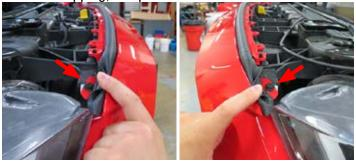
6. (Fig. 1) On Performance Package Vehicles, Remove eight (8) push pins securing the splash guard using a panel puller. (Fig. 2) For all other models, remove six (6) push pins. The splash guard will be removed with the bumper.
