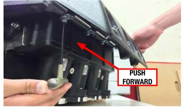
57. Using O-ring lube, install the fuel caps onto the fuel rails. Attach the supplied fuel crossover to the rear of both rails. Insert the straight fittings into the fuel rails as shown.
