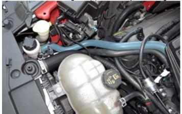
96. Using a 10mm socket, remove the top bolt securing the windshield wiper fluid reservoir. Place the surge tank bracket onto reservoir and secure the bracket and reservoir using the factory bolt.
