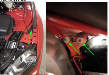
10. From within the wheel well remove the fascia retention assembly that the nuts were removed from in the previous step. Pull downward until the until the plastic pin no longer retains the assembly. Remove from vehicle, ensuring to distinguish between passenger and driver side.
