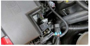
100. Open the fuse box and using a 10mm socket, attach the "Power Supply Wire" on the Water Pump/EVAP Harness to the power terminal on the fuse box.
