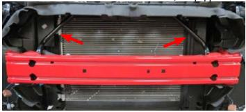
85. Back out the four (4) crash beam bolts (circled in image) but do not remove. Install the LTR brackets from behind the crash beam and onto the crash beam support studs. Line up the holes on the LTR brackets with the studs to temporarily hold the LTR brackets in place. Then install the LTR from below as pictured.
