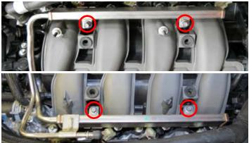
34. Using an 8mm socket, remove six (6) manifold bolts.
