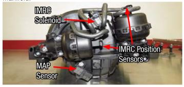
36. Make sure the IMRC harness is completely disconnected from above locations and remove the manifold. Clean the cylinder head flanges as needed and tape up the ports to prevent debris from falling into the ports. **NOTE:** Adjust the upper radiator hose clamp position to point more towards the driver's side of he vehicle. The supercharger housing will be occupying this space later. (See arrow)
