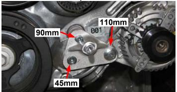
47. Install and secure the 76mm idler pulley onto the center of the idler bracket by using the M8 Washer and the M8 x 20mm bolt supplied in Bag # 2 using a 12mm socket. Use blue thread lock fluid on the bolt threads and torque to 18 ft-lbs.
