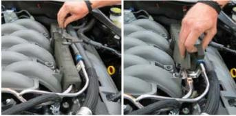
30. Disconnect eight (8) fuel injector connectors.
